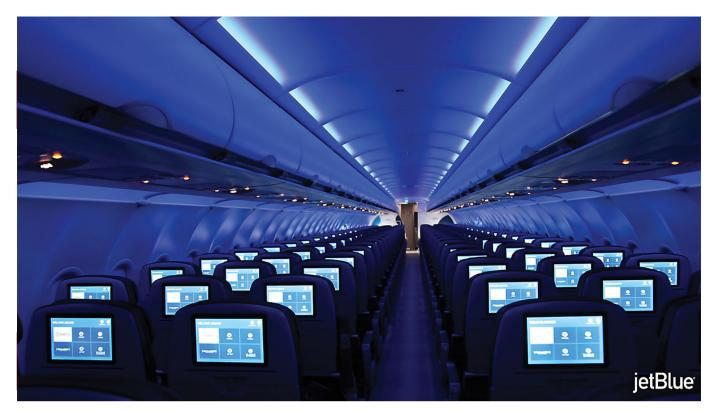
Above: LED cabin lights, which can be programmed to shift in brightness, warmth, and colour throughout the flight, have become common on new planes.
